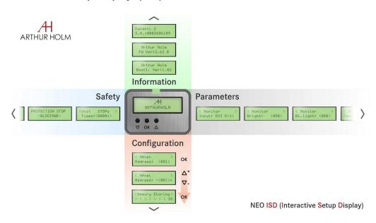
Screen to configure the monitor address in the RS422 AHnet.
