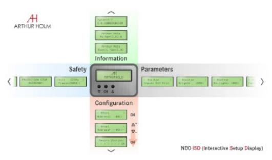
Screen to configure the monitor address in the RS422 AHnet.
