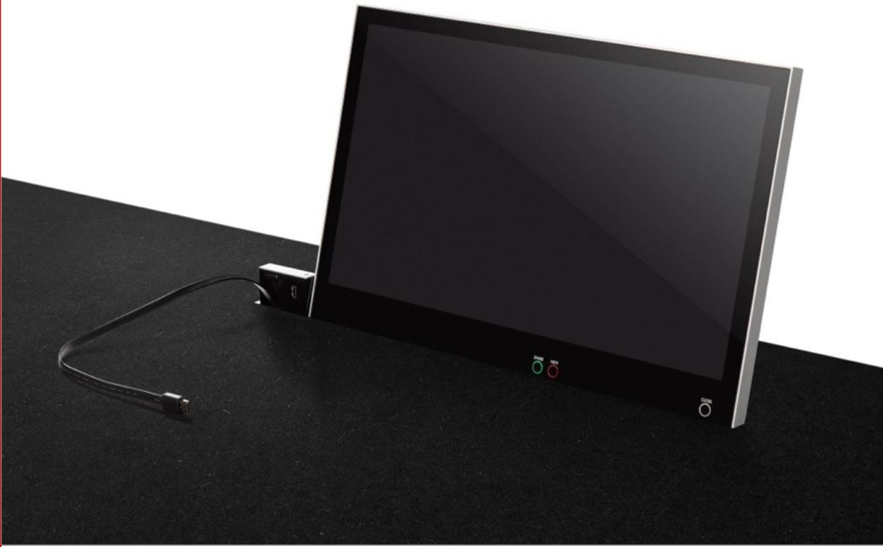
The View and Share buttons are placed on the monitor's front glass, so the user can easily select the input (View) and share it (Share).
